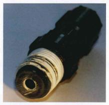
**WITH CHLOR-FLOW** in the chlorine solution, under similar water conditions, this assembly had been in operation for 180 days of uninterrupted service.
