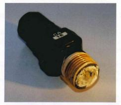
This chemical metering pump injection assembly was used in pumping a chlorine solution **WITHOUT CHLOR-FLOW**. After only 30 days, scale deposits made chemcial injection impossible.
